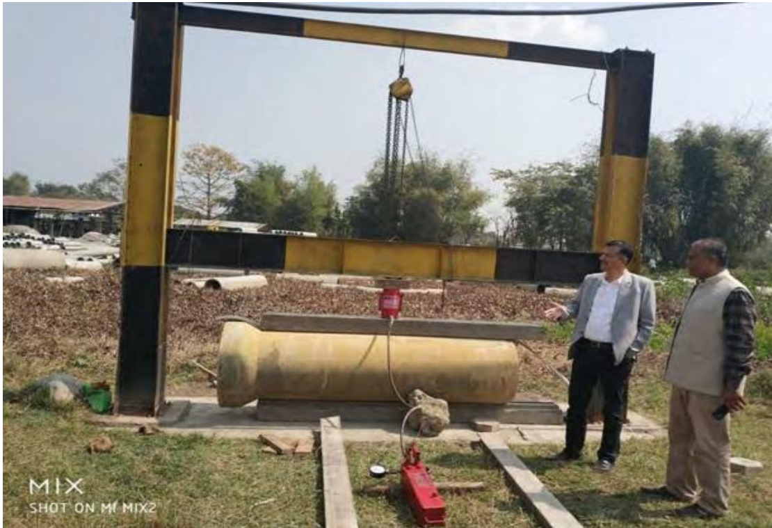
Three Edge bearing Test of Hume/RCC pipe, Biratnagar
