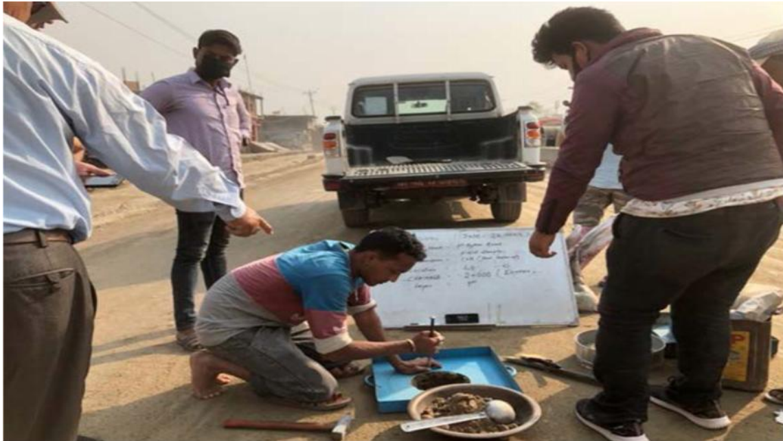
Conduction of Field Density tests of Base course, Birgunj
